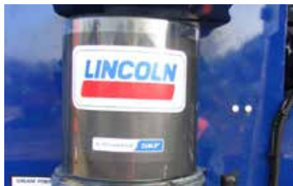
Central Auto-lube System - ensure against excessive component wear
