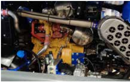
Tier 4 Final / STAGE V - CAT3.6 100Kw (134HP)
