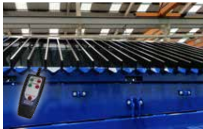
Reject Grid - manual or remote tipping grids available with various bofor bars
