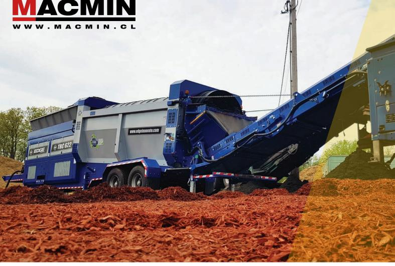
With unmatched production rates of 500 yards<sup>3</sup>/hr and high efficiency; the EDGE ColorPRO offers operators the highest return of any coloring system available on the market. A self-contained portable coloring system, the EDGE ColorPRO is ideal for those operators seeking a large capacity, coloring solution.
