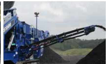
Fines Discharge Conveyor
